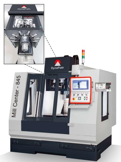
The DynaPath WinDelta control system enables the machine to be operated manually in DRO Mode, by teaching positions and commands in the Semi-Auto Mode, or by running G-Code programs in full Auto Mode. Programs can be created with the built-in Conversational + DXF Editor, or by direct G-Code programming.
